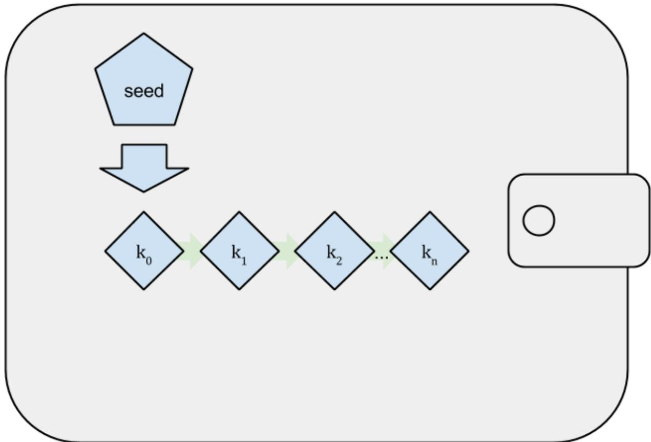
Figure 27. Type-1 deterministic (seeded) wallet: a deterministic sequence of keys derived from a seed
