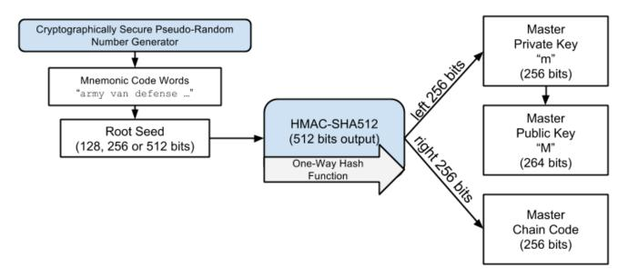
Figure 34. Creating master keys and chain code from a root seed
