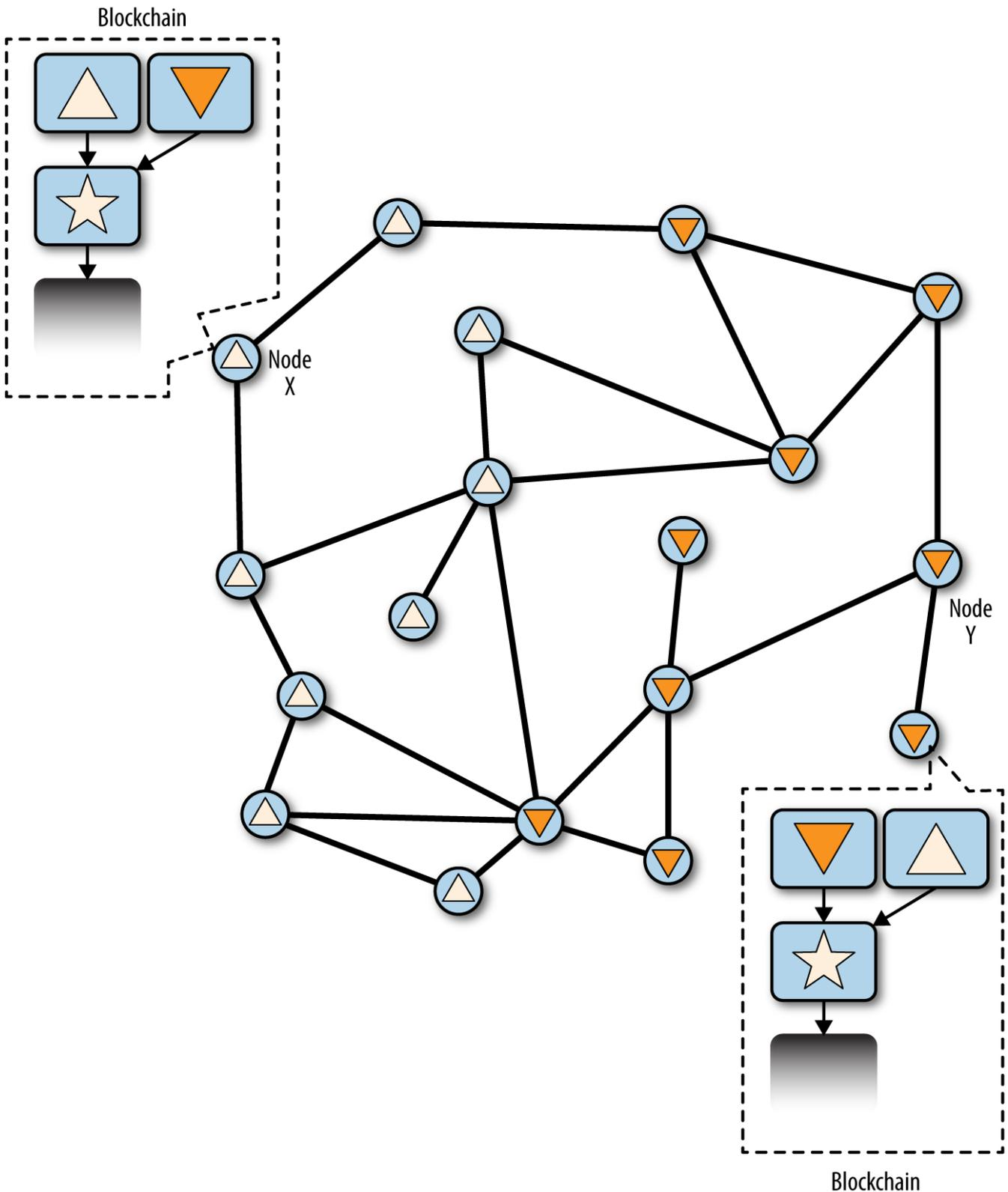
Figure 68. Visualization of a blockchain fork event: two blocks propagate, splitting the network
