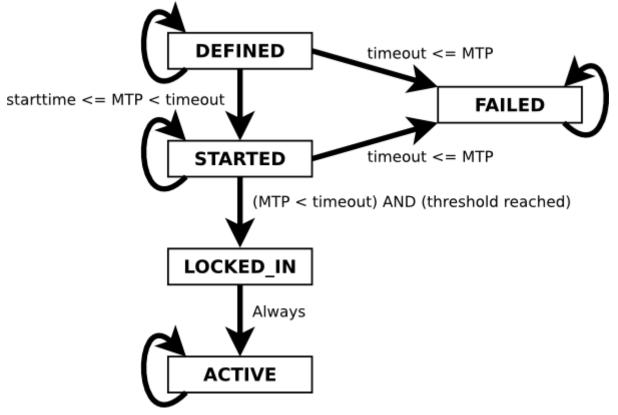
Figure 74. BIP-9 state transition diagram
