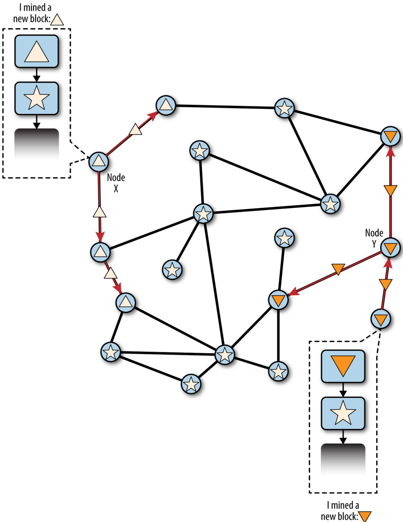
Figure 67. Visualization of a blockchain fork event: two blocks found simultaneously
