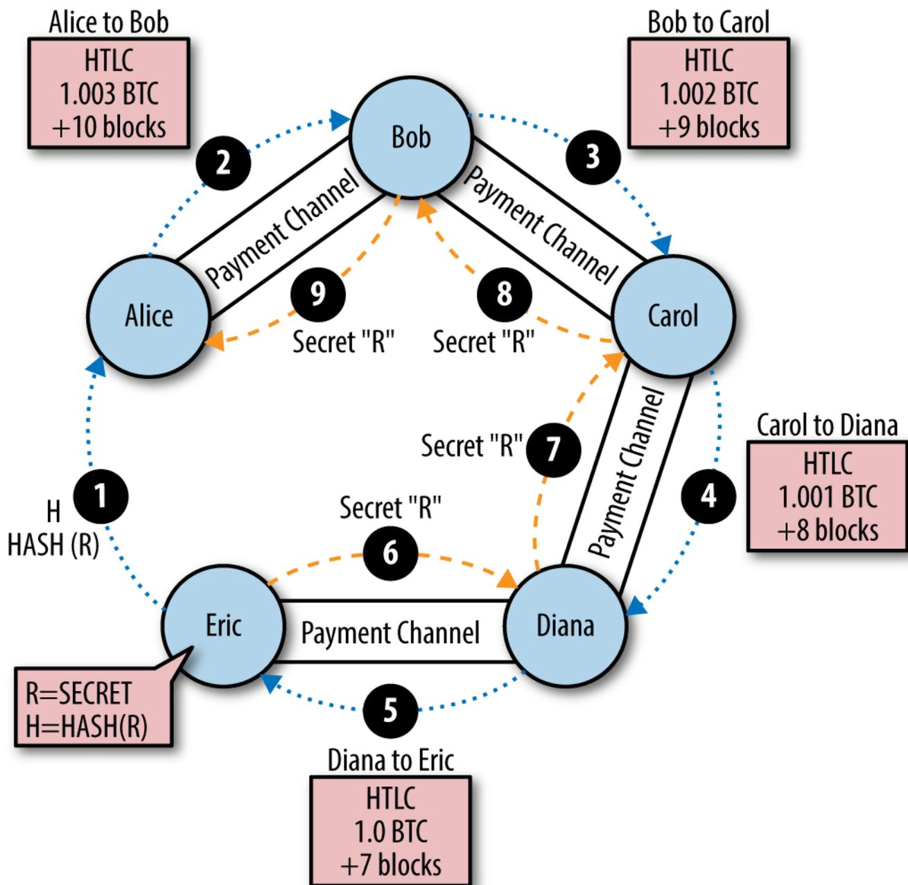
Figure 84. Step-by-step payment routing through a Lightning Network
