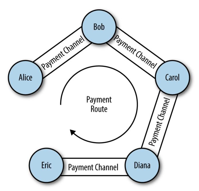
Figure 83. A series of bidirectional payment channels linked to form a Lightning Network that can route a payment from Alice to Eric
