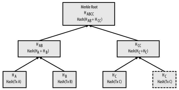
Figure 62. Duplicating one data element achieves an even number of data elements
