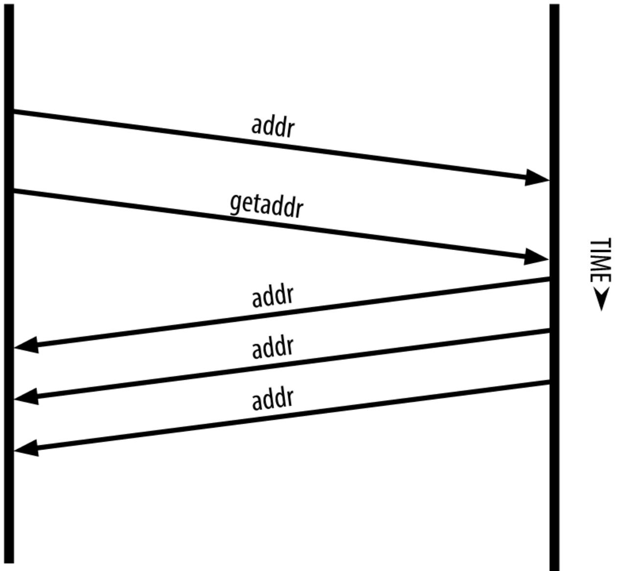
Figure 52. Address propagation and discovery
