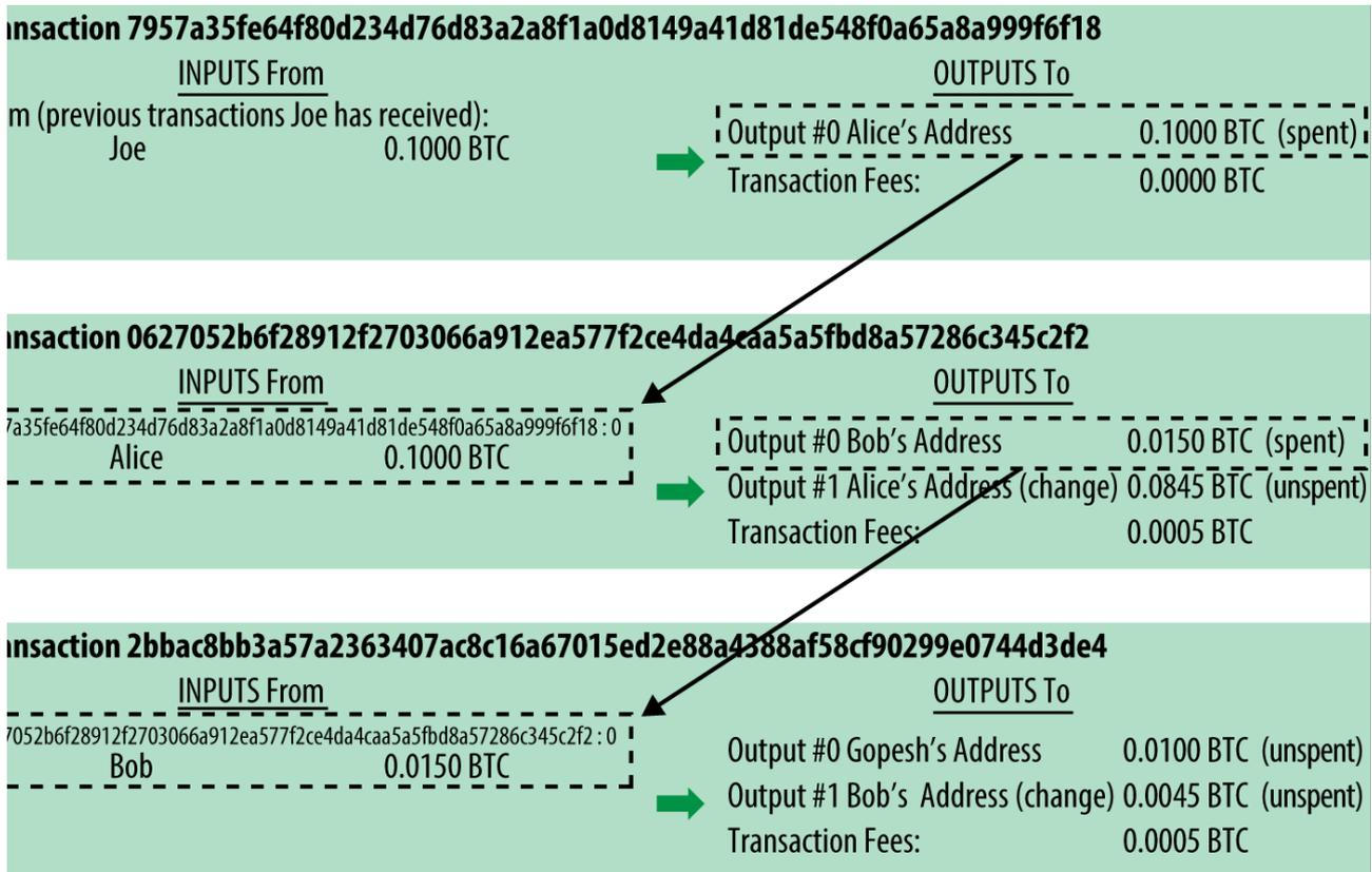
Figure 6. A chain of transactions, where the output of one transaction is the input of the next transaction
