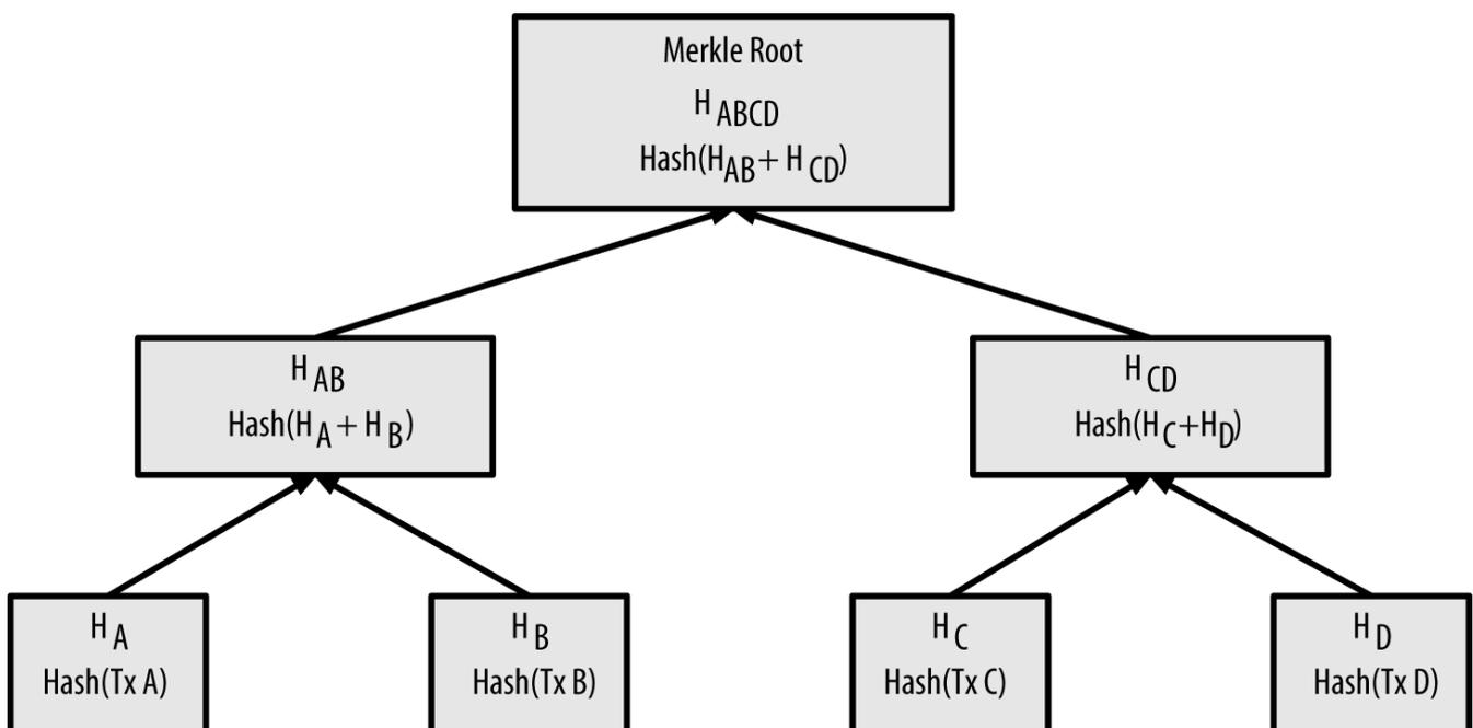
Figure 61. Calculating the nodes in a merkle tree
