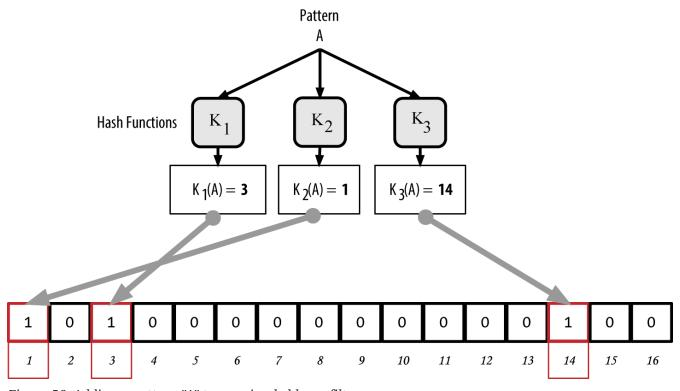
Figure 56. Adding a pattern "A" to our simple bloom filter
