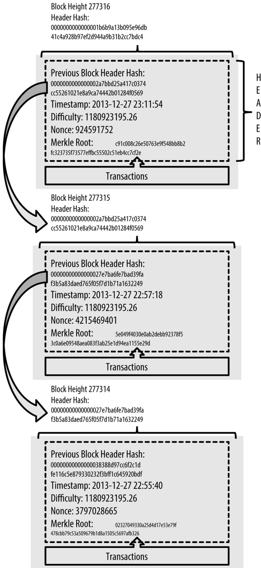
Figure 60. Blocks linked in a chain by reference to the previous block header hash
