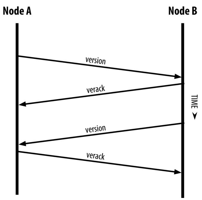
Figure 51. The initial handshake between peers
