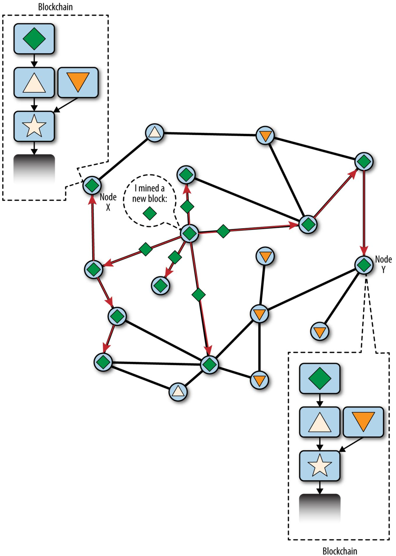
Figure 69. Visualization of a blockchain fork event: a new block extends one fork, reconverging the network
