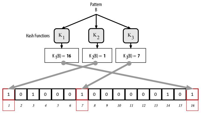
Figure 57. Adding a second pattern "B" to our simple bloom filter
